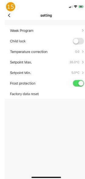
Basic settings such as the minimum and maximum temperature, the childproof lock, frost protection and the weekly programme (Fig. 16) can be set by tapping 'Setting'.
