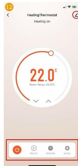
The picture shows the main view of the thermostat. The target temperature (setpoint) is displayed in the centre and the current room temperature is displayed below it. The setpoint temperature can be adjusted manually using the arrow buttons. The functions of the 'Switch', 'Mode', 'Schedule' and 'Setting' buttons are explained in Figures 13, 14, 17 and 15.
