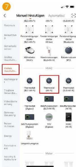
To integrate a thermostat, tap on 'Small household appliance' on the left and then select 'Thermostat (Wi-Fi)' on the right. Do not select Bluetooth, Zigbee, BLE+Wi-Fi!
