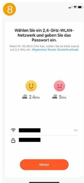
Select the WLAN network (SSID) of the existing router and enter the corresponding WLAN password.
