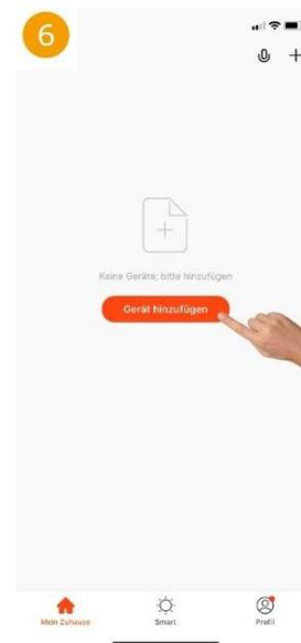
The thermostat can now be integrated by tapping on 'Add device'.
