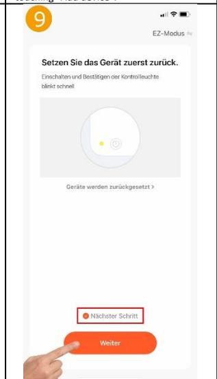
Set the thermostat to teach-in mode: Press the on/off key on the thermostat for approx. 3 seconds until "11" appears on the display (if necessary, unlock the keys first). Now briefly press the "+" key, the "11" should now flash and the thermostat is in teach-in mode. Now in the app first tap on "Confirm indicator rapidly blink" and then on "Next".
