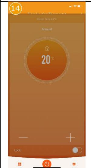
The thermostat can be switched off or on by touching the "switch" symbol in the middle at the bottom of the main thermostat display.
