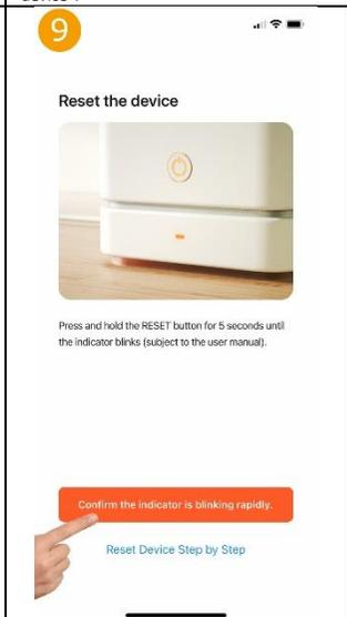
Set the thermostat to teach-in mode: Press the down arrow button on the right of the thermostat for approx. 3 seconds until the WLAN symbol flashes quickly in the upper right corner of the display. Now in the app tap on "Confirm the indicator is blinking rapidly".
