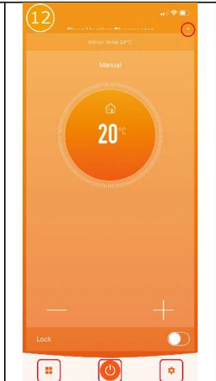
Main view: The setpoint temperature is displayed in the middle and the current room temperature (Indoor Temp) above it. The setpoint temperature can be adjusted manually using the Plus/Minus button. The key lock can be switched on/off using the "Lock" key. Functions of the other buttons see 13, 14, 15, 18.
