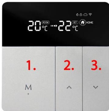
1. 1. mode & on/off key, short key press change operating mode, long key press (3 sec.) on/off.
