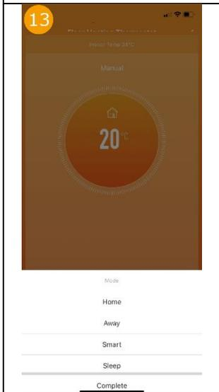
Tap the "Mode" icon in the lower left corner of the main thermostat display to change the thermostat operating mode (Home/Away/Smart/Sleep).
