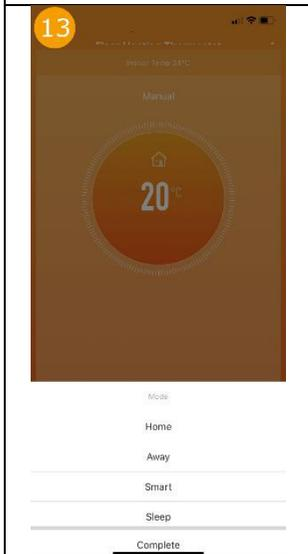
By tapping the "Mode" icon at the bottom left of the main view of the thermostat, the operating mode of the thermostat can be changed (Home/Away/Smart/Sleep).
