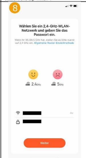
Select the WLAN network (SSID) of the existing router and enter the corresponding WLAN password.
