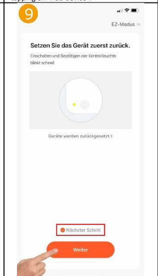
Set the thermostat to teach-in mode: Switch off the thermostat and press the Eco button (button 3) for approx. 5 seconds until the Wifi symbol appears in the display. Now tap on 'Next step' in the app and then on 'Next'.
