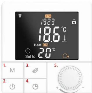
1. Mode button, short button press Change operating mode, long button press (5 sec.) Programming weekly programme
