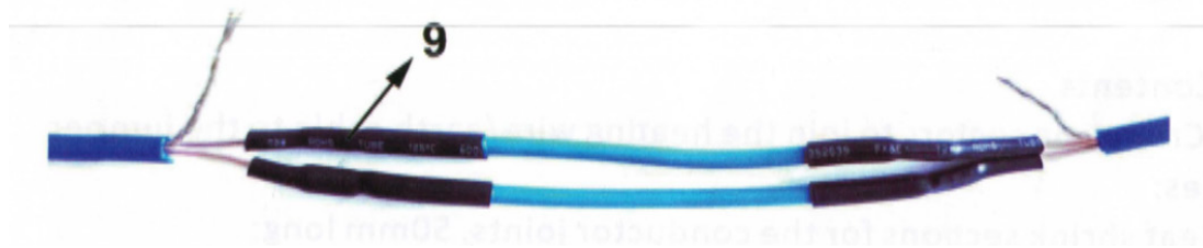
Step 9 - heat-shrink tubing over the individual conductor connections. Schematic illustration.
