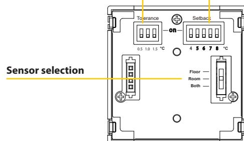
Remove the front shell. Three DIP switches are marked with temperature tolerance, setback, and sensor options respectively. The following pictures describes how to set the parameters.
