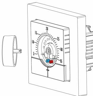
Place the red and blue pins in the holes of the array in the figure to set the temperature range you want. For example, place the knob pointer in the range of the red and blue pins in the figure, which means that the adjustable temperature is 10-20°C.
