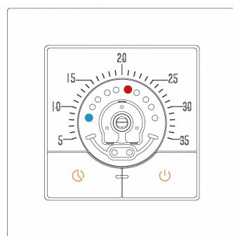
When installing the knob, take care to install the pointer position marked on the knob to the middle of the red and blue limit pin. In this way, the knob is limited to a range of 10-20° rotation.
