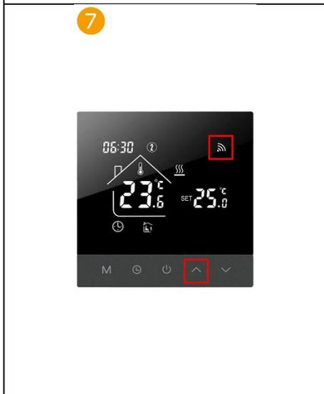
Set the thermostat to teach-in mode: Switch on the thermostat and press and hold the ▲ button for approx. 5 seconds until the WLAN symbol flashes on the thermostat display.
