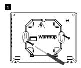
Insert fixing screws through mounting holes of the power module and tighten.
