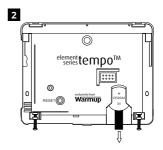
Locate your CR2032 3-Volt lithium battery on the reverse of the front housing. Remove the plastic strip from under the battery. The battery should always be installed with positive side "+" facing outwards.
