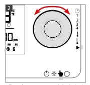
Turn the rotary control clockwise/ anti-clockwise to increase or decrease the target temperature
