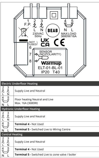
For extra low voltage or volt-free systems a contactor must be used. Connecting the tempo directly to extra low voltage or volt-free boilers may cause damage to the boiler circuit.
