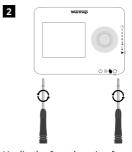
Unclip the front housing from the power module.
