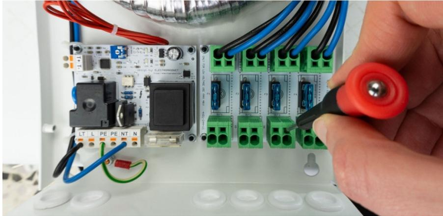
The transformer can be switched either via 230V mains voltage or via a potential-free switching contact. Depending on the selected switching variant, the temperature switch installed in the toroidal core (red connection lines) must be wired.
